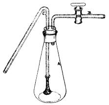
In this finnel is placed a wad of glass-wool. Tubes and stoppers must fit airtight into the flask. The apparatus is accurately tared; from three to four grammes of pure grape sugar in small pieces are then placed in the flask. fifteen to twenty c. c. of a 40%, caustic soda solution, sixty c. c. of water, and sufficient 90%, alcohol (120 c. c.) to bring the whole to about seven
